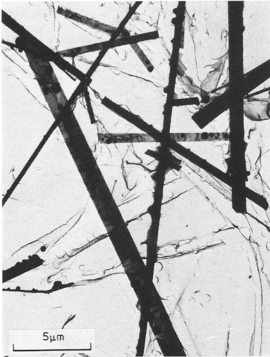
Figure 7 Nickel particles and sapphire whiskers after 2 h at 1300°C.
