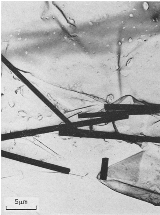
Figure 1 Uncoated sapphire whiskers after 17 h at 1300°C.
