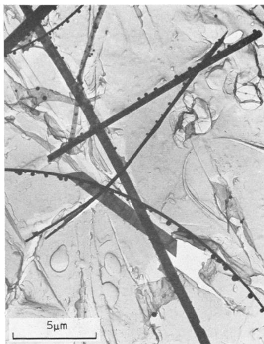
Figure 6 Nickel particles and sapphire whiskers after 2 h at 1200°C.
